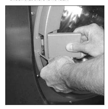
■ First position the screwdriver in the opening, then push it in and hold it securely.
