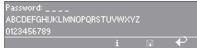
After keying in your password or inserting your supervisor level key card in the reader the following security prompt will appear in the display:
