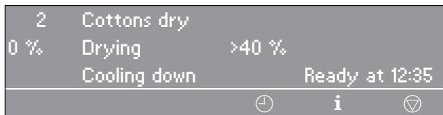
In the 2nd line of the display, drying in this example, the actual residual moisture level (>40%) will also be shown. The 3rd line displays the following programme block.
