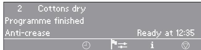
The programme end time is displayed, the buzzer sounds and the anti-crease phase commences. The drum will rotate at intervals to keep the laundry from creasing.
