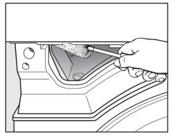
Use a bottle brush to remove detergent residues and limescale from the jets inside the detergent dispenser drawer housing.
