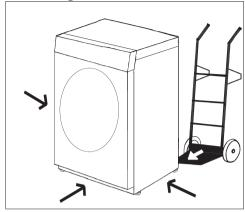
■ Transport the machine to its installation site.
