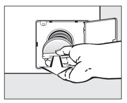
■ Remove the drain filter completely.
